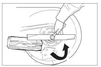
Figure 24. Loosening the Mower Blade for Removal
